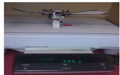
(c) Weighs approx. 98.6 grams with PID controller, camera, brushless motor, Li-PO battery and wings.
