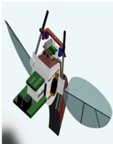
(a) The CAE SolidWorks model of the recently designed Bumblebee MAV.
